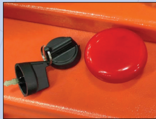
Key switch prevents unauthorized use; Emergency e-stop halts operation
