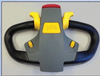
Ergonomic handle with left/right hand controls and "belly bump" switch
