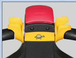
Turtle-speed button reduces drive speed by 50% for precise positioning
