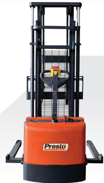
Telescopic Mast Straddle Lift Heights up to 150"
